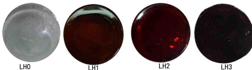
Figure 1. Representative photographs of hydrogels with different EOL content (LH0, LH1, LH2, and LH3). [Color figure can be viewed in the online issue, which is available at wileyonlinelibrary.com .]
